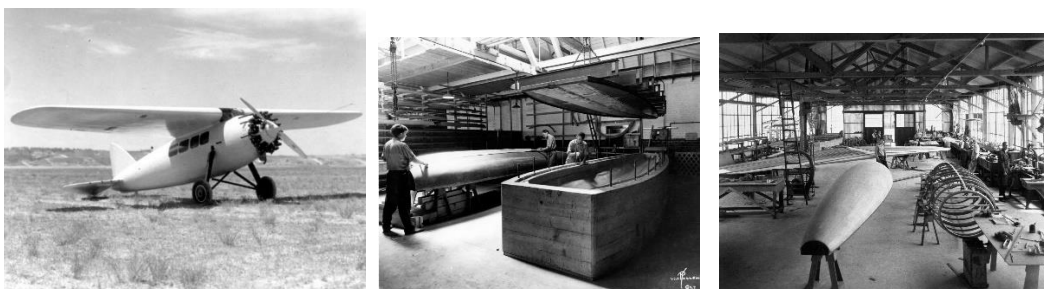
Figure 66: The Lockheed Vega, the concrete molds used to form the fuselage halves and components of the first Lockheed Vega 1 before assembly (Reproduced from [11])
