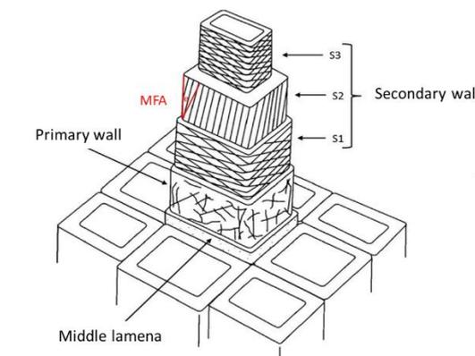
**Figure 7 - Schematic of a wood cell [31].**
