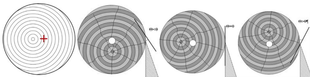
**Figure 25 – Representation of an eccentric log [59]**
