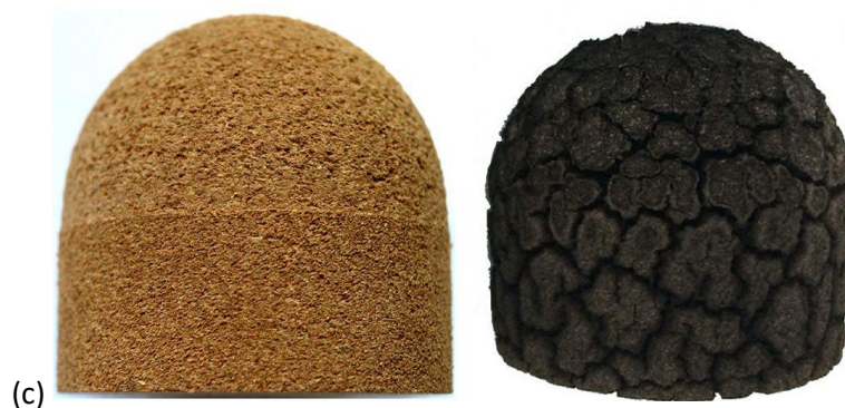
Figure 73: (a),(b) views of the Schiaparelli Front and Back Heat Shield TPS during assembly. Copyright: Airbus Defence and Space SAS 2014 A. Gilbert. The images are available on the ESA Exploration web site http://exploration.esa.int/ ; Reproduced from [267]. (c) The transformation of cork in charts after a burning test with a plasma torch (reproduced from [269]).
