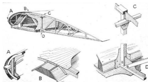
**Figure 65: Typical design of a wood wing and internal joints (reproduced from [7])**
