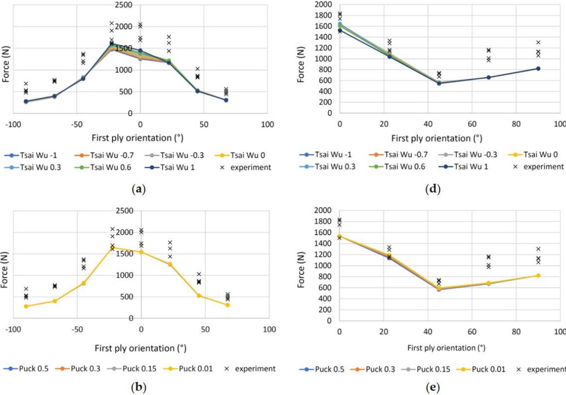
**Figure 41 – Failure forces measured and calculated on 7-ply specimens (7A and 7P) LVL loaded in 4-point bending: (a) 7A specimens, Tsai-Wu criterion; (b) specimens 7A, Puck criterion; (d) 7P specimens, Tsai-Wu criterion; (e) 7P specimens, Puck criterion [131, 132]**
