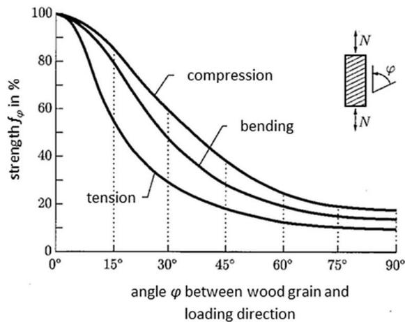
**Figure 31 – Schematic curves of the loss of strength of wood in tension, bending and compression as a function of the angle  $\varphi$  between the fibers and the direction of the loading  $\vec{N}$  [26].**
