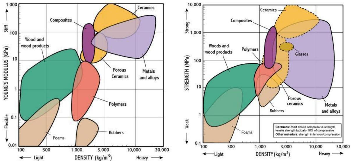
**Figure 10: modulus–density chart for common mechanical construction materials (left) and strength-density chart (right) [39].**
