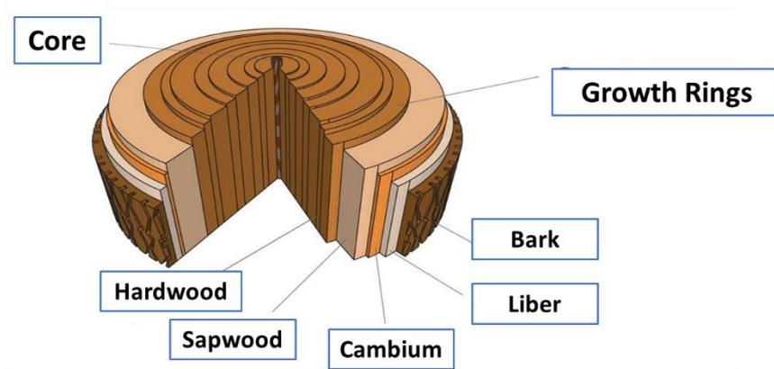
**Figure 6 – Cross section of a tree trunk.**
