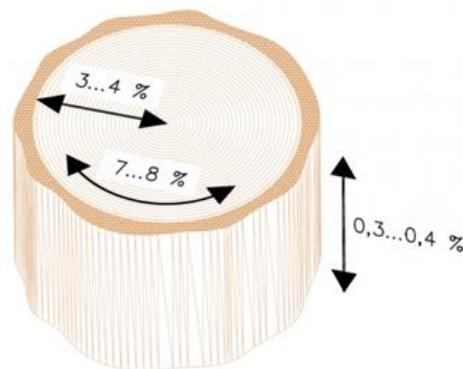
**Figure 15– Shrinkage values as a function of wood direction [29]**
