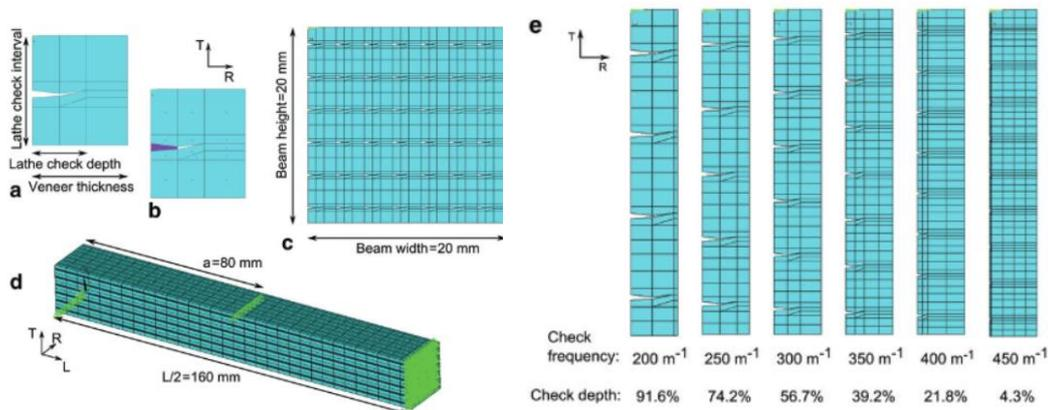
**Figure 39 – Finite element model of an LVL beam. (a) Base Pattern; (b) base pattern with glued cracks (the glue is purple in color); (c) beam cross-section (crack frequency  $300\ m^{-1}$ ); (d) half of the beam (the green triangular symbols represent the boundary conditions); (e) finite element model of the six cracked veneers used in the numerical model [120].**
