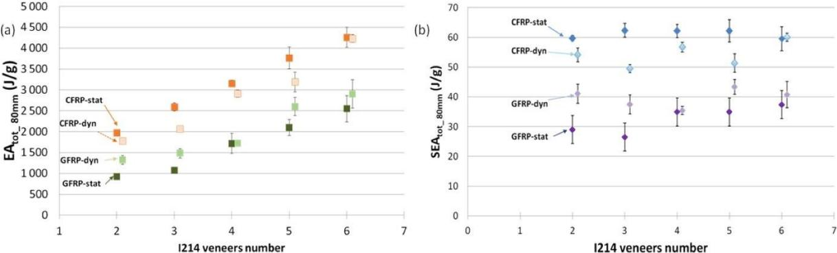
**Figure 47. Evolution of (a) EA<sub>tot\_80 mm</sub> (b) SEAtot<sub>80 mm</sub> according to the number of poplar layers, the nature of the skins (CFRP: Carbon Fiber Reinforced Polymer; GFRP: Glass Fiber Reinforced Plastic), and static and dynamic conditions. Reproduced from [199]**
