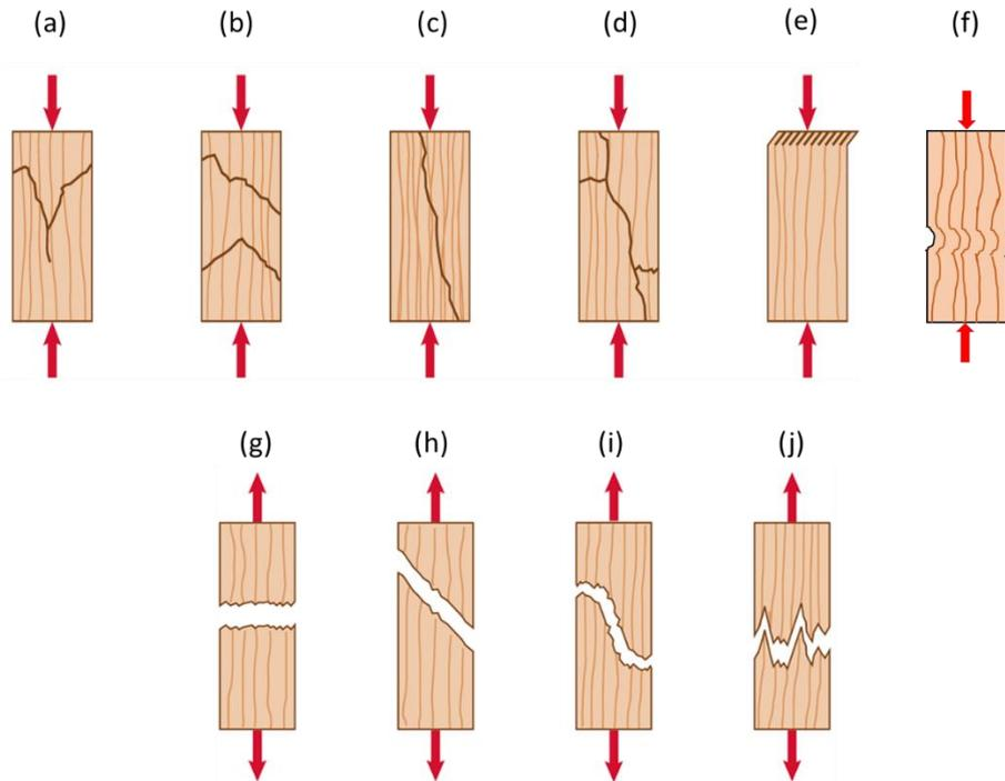
**Figure 9 – Failure in longitudinal compression: (a) failure by fiber crushing, (b) bevel splitting, (c) simple splitting, (d) splitting by transverse failure, (e), extremities crushing, and (f) kinking. Failure in longitudinal tension: (g) pure tension, (h) shearing, (i) tension + shearing, (j) tension + splitting**
