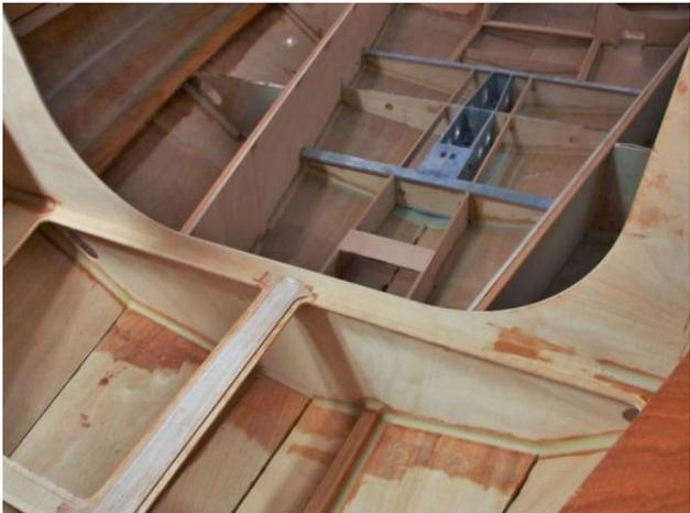
**Figure 55: Plywood structure of an RM sailboat [219]**
