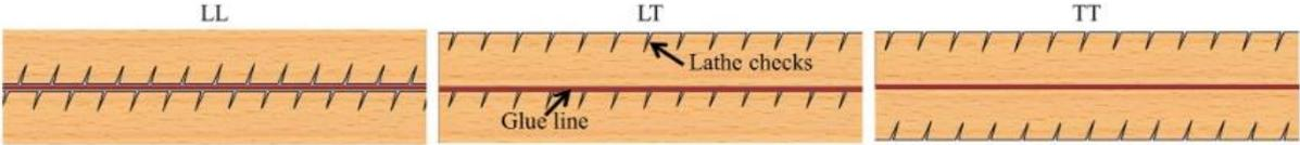
**Figure 28 – Three different LVL bonds for shear tests [71]**
