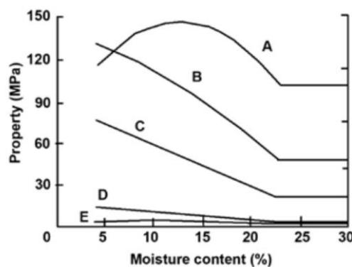
**Figure 13 - Effect of moisture content on the strength properties of wood. A: tension parallel to the grain; B: bending; C: compression parallel to the grain; D: compression perpendicular to the grain; and E: traction perpendicular to the wire [32].**
