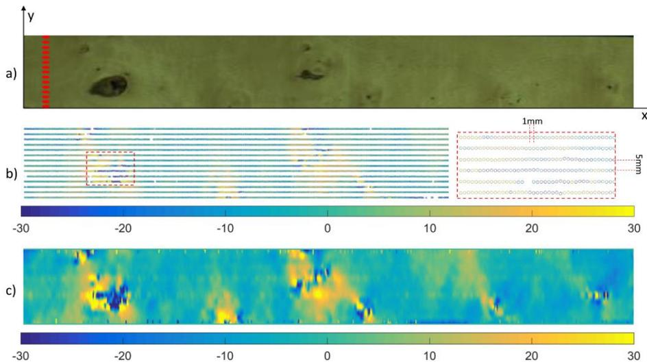
**Figure 36 – Local grain angle measurement: (a) photograph, (b) raw data, and (c) interpolated data [113]**
