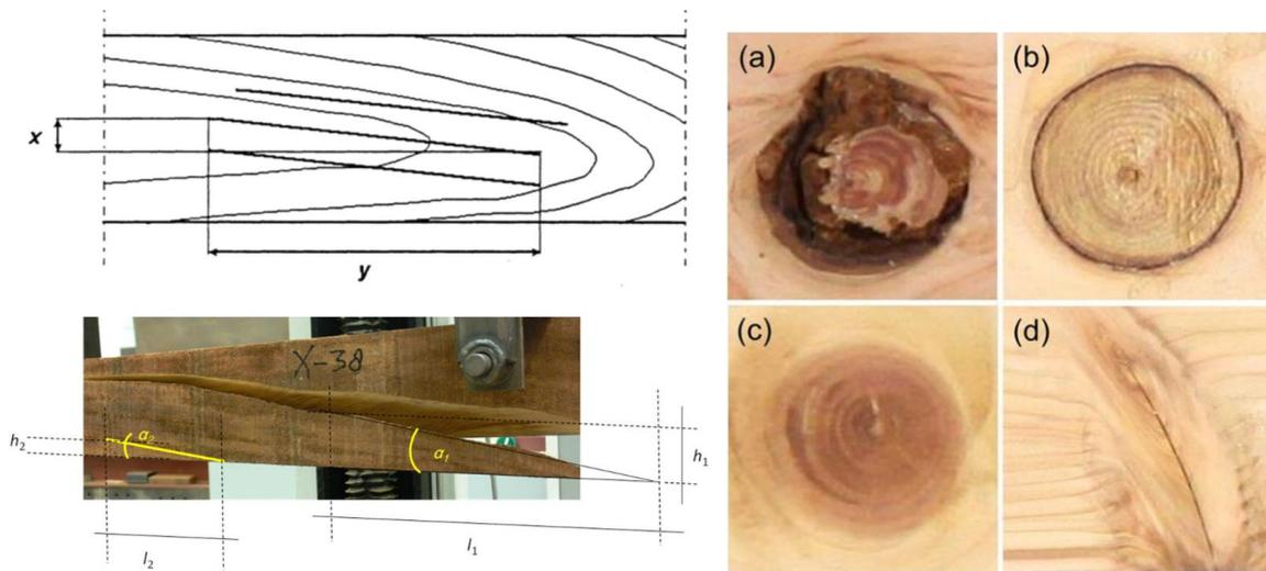
**Figure 19 – Left: Definition of the slope of the grain according to standard EN 1310 (Top), Angle of the grain and associated slope of the fiber angle measured during a bending test (Bottom). Right: Four types of wood knots: (a) rotten knot, (b) coated knot, (c) sound knot (d) sharp knot [49, 50].**
