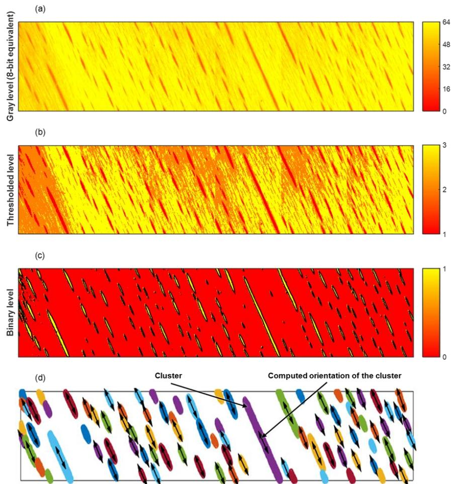
**Figure 37 – Image processing state during the grain direction computation: (a) initial image (grayscale converted to 8-bit), (b) 3-level thresholded image, (c) binarized image on which medullar rays contours were detected and drawn (black contour), and (d) clusters and their main directions indicated by the corresponding double-arrow. Clusters where no arrow is associated were not considered in the computation (area too small or shape not elongated enough (Reproduced from [114]))**
