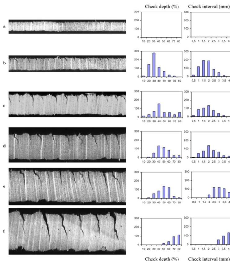
**Figure 26 – Lathe checks on beech veneer of different thicknesses: 0.7 mm (a), 1.0 mm (b), 1.5 mm (c), 2.0 mm (d), 2.5 mm (e), 3.0 mm (f), presented with histograms (number of control occurrences on a 1 m long veneer) of control depths per turn (in % of the thickness) and intervals [65].**
