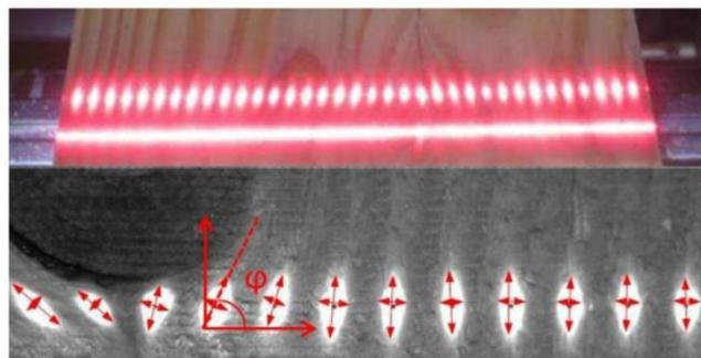
**Figure 35 – Tracheid effect by projection of a laser beams line over a Douglas fir beam surface. Example of grain angle deviation around a knot [48]**
