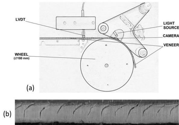
**Figure 34: (a) SMOF, optical lathe check measuring system (LVDT = linear variable differential transformer) Erreur ! Source du renvoi introuvable., and (b) an image of Douglas fir veneer obtained with it**
