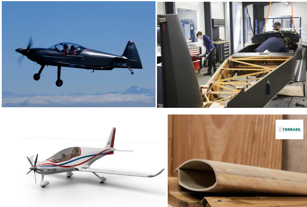
Figure 71: Two new wooden light aircraft in France: Aura aero Integral R and its carbon-wood structure and the forthcoming “Avion Mauboussin” and a picture of a wing made with a wood-based sandwich “YGDRASIL”.
