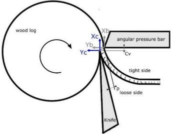
**Figure 21 – Schematic diagram of the process for peeling a wooden log.**
