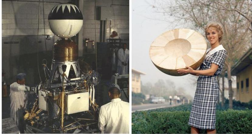
**Figure 72: Rangers 3, 4, and 5 each had a seismometer encased in balsa wood to limit the impact loads for moon exploration (1962), [263].**
