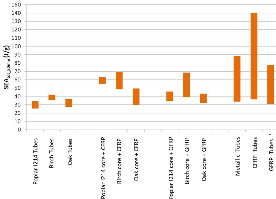
**Figure 48. SEAtot\_80mm for the wood species tested and for others materials (Reproduced from [202]).**
