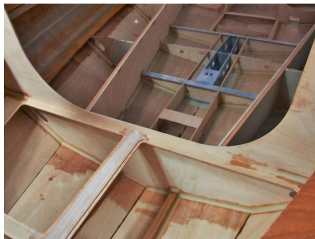
Figure 55: Plywood structure of an RM sailboat [219]
