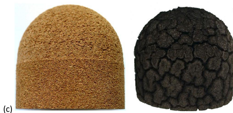
Figure 73: (a),(b) views of the Schiaparelli Front and Back Heat Shield TPS during assembly. Copyright: Airbus Defence and Space SAS 2014 A. Gilbert. The images are available on the ESA Exploration web site http://exploration.esa.int/ ; Reproduced from [267]. (c) The transformation of cork in charts after a burning test with a plasma torch (reproduced from [269]).
