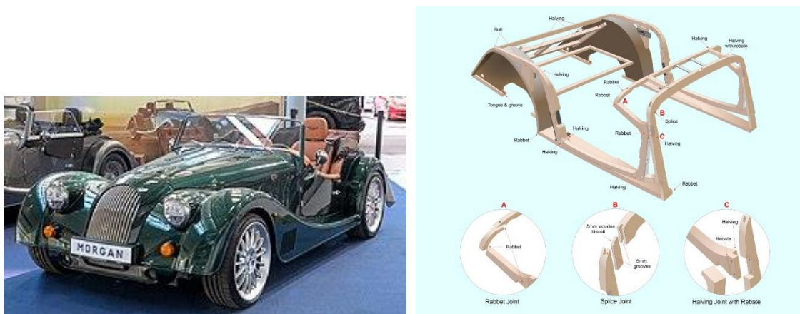
Figure 61: The last model of Morgan cars, the "Morgan Plus Six" and its ash frame structure [231, 233].
