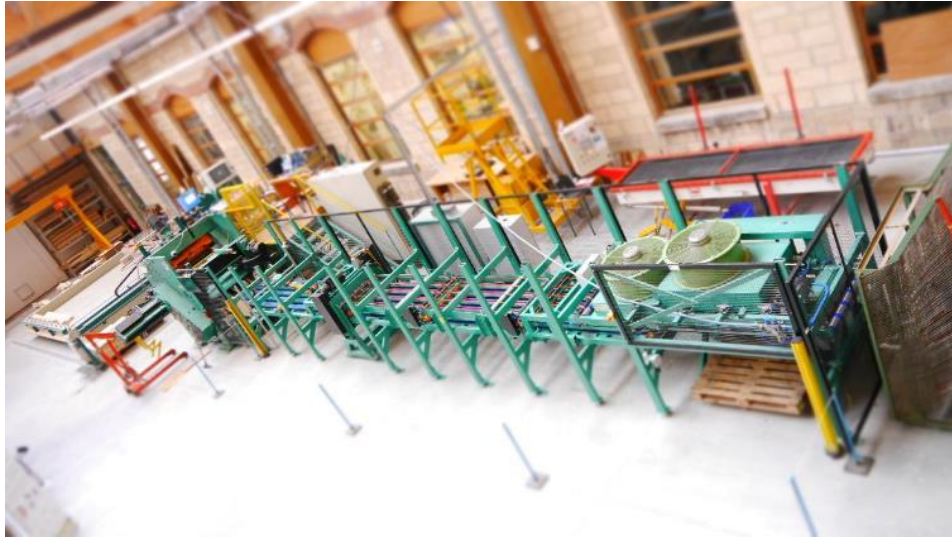
Figure 22 – logwood peeling platform, LaBoMaP (Arts et Métiers, Cluny, France)
