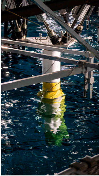
Fig. 5. Installation of captive platform model, where the rigid connection between the model platform in yellow and the hexapod (not visible here).
