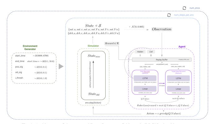
Fig. 1: Architecture of the proposed Deep Recurrent Q-Network (DRQN) algorithm
