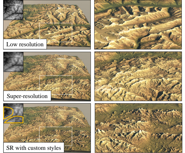
Figure 12. A 90 km terrain of 30 m precision was obtained with the super-resolution tool (center) from an initial low resolution model (top). We controlled the generation by adding iteratively two different styles (bottom).
