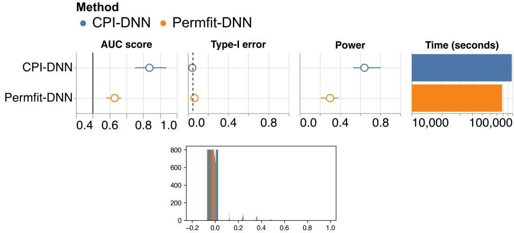
Figure E3: Semi-simulation with UK Biobank: (Top panel) Performance of CPI-DNN and Permfit-DNN is compared in terms of AUC score , Type-I error , Power and Time on the data from UKBB with n = 8357 and p = 671 . (Bottom panel) Correlation strength among the variables in the UKBB dataset.
