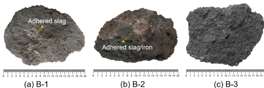
Fig. 11. Post-mortem castables delivered from locations in the middle of the runner, slag line B-1 (a); slag/iron line: B-2 (b), iron line: B-3 (c).
