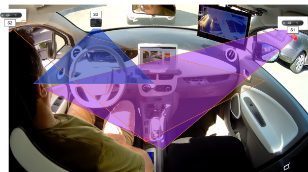
Fig. 3. Acquisition module setup: Sensors S1 and S2 capture a lateral view of the scene (Intel Realsense D435 cameras), and sensor S3 captures a front view of the upper body (GoPro model 8). Domain-specific data, such as internal states and attitudes towards the SDC, are acquired using surveys that are applied before, during and after vehicle usage.
