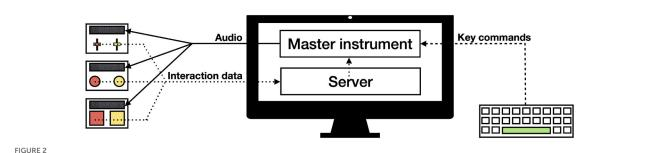
The system with three instruments sending control data (OSC) to a Node.js-server. The data is forwarded to the master instrument (in a web client). The instrument data is combined with the master instrument interactions to determine the audio output sent to the loudspeakers of respective
