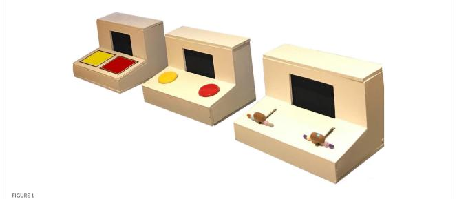
The three Funki instruments used in the study, with different controllers. From the left: two touch-sensitive pads, two momentary buttons, and two sliders. The black area is the backside of the loudspeaker.
