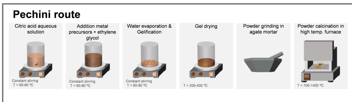
Figure 5: Illustration of the steps involved in the Pechini route
