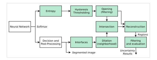
Fig. 3: Block diagram of an application detecting regions with high uncertainty in a segmented image.
