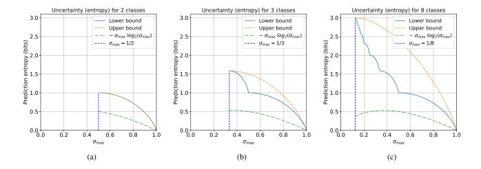
Fig. 1: Upper and lower bounds of entropy against the probability of the predicted class and the partial contribution of  $\sigma_{max}$  to entropy for segmentation with 2 (a), 3 (b) and 8 (c) classes
