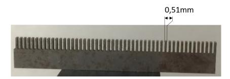
Figure 13: Calibration comb prototype with 0.51 mm teeth width
