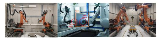
Figure 1: X-Ray CT robotic cell including industrial robots located on tracks [10] [11] [12]
