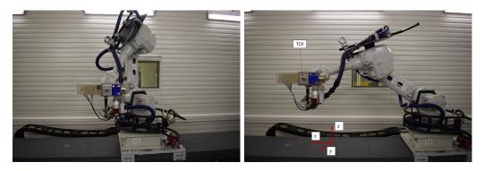
Figure 5: Linear trajectory measurement from folded (a) to stretched (b) arm configurations
