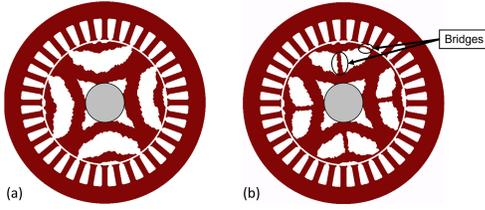
Fig. 4. Magnetic (a) and mechanical (b) optimization result.
