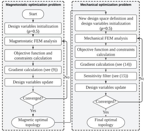
Fig. 2. Flowchart of the proposed two-step optimization procedure.
