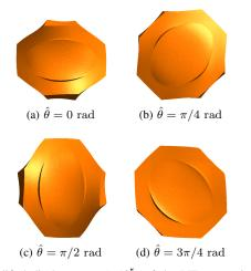
Fig. 6. Amplified displacements (×10<sup>5</sup>) of the ME composite for angles  $\hat{\theta} = 0, \pi/4, \pi/2 \& 3\pi/4$  rad, top view
