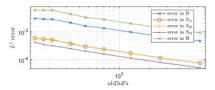
Fig. 1.  $L^2$  error of the magneto-mechanical solutions compared to the analytical solutions vs the number of total DoFs of the magneto-mechanical problem.
