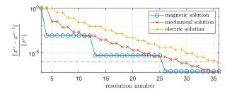
Fig. 3. Convergence of the single-physics solutions in generator mode within the multi-physics solver for the ME generator at  $\hat{\theta} = 0$  rad.
