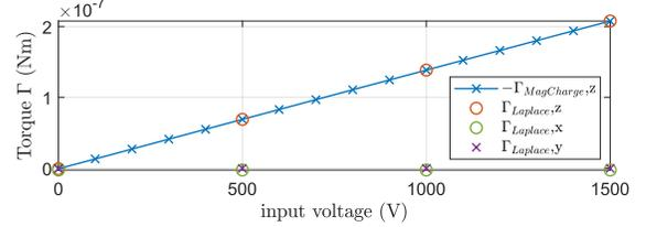
Fig. 4. Global torque  $\Gamma$  between the Galfenol disk and the magnet vs the voltage applied to the piezoelectric layer. It is computed as a Laplace force in the magnet, and its (z) component is compared to the torque computed by the magnetic charge method in the Galfenol layer.
