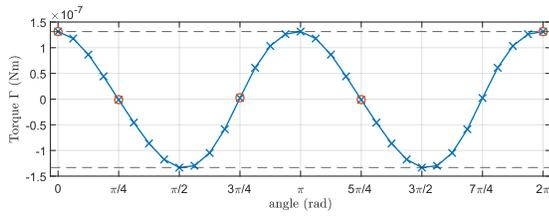
Fig. 5. Torque  $\Gamma$  vs rotation angle  $\hat{\theta}$ . Cross markers correspond to the z-component of the torque in the Galfenol layer ( $-\Gamma, z$ ), circle markers correspond to the z-component of the torque in the magnet, for 33 angles  $\hat{\theta}$  describing the full rotation of the magnet.
