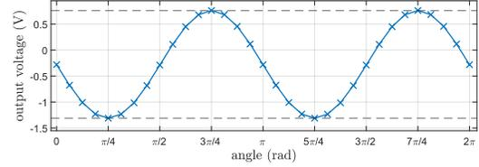
Fig. 7. Potential difference between the reference electrodes,  $e_1$  and  $e_2$ , and the floating potential electrodes,  $e_3$  and  $e_4$ , vs the angle  $\hat{\theta}$  between the magnet and the ME composite.
