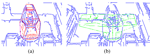
Fig. 22: Super-imposition between projected edgelets from the current state (red) and 2D image contours (blue) on the left, and between projected edgelets from a false potential state (green) and 2D contours on the right. To estimate the accurate state of the valve, false positive association as between edgelets from the potential state and the static part of the object have to be considered.
