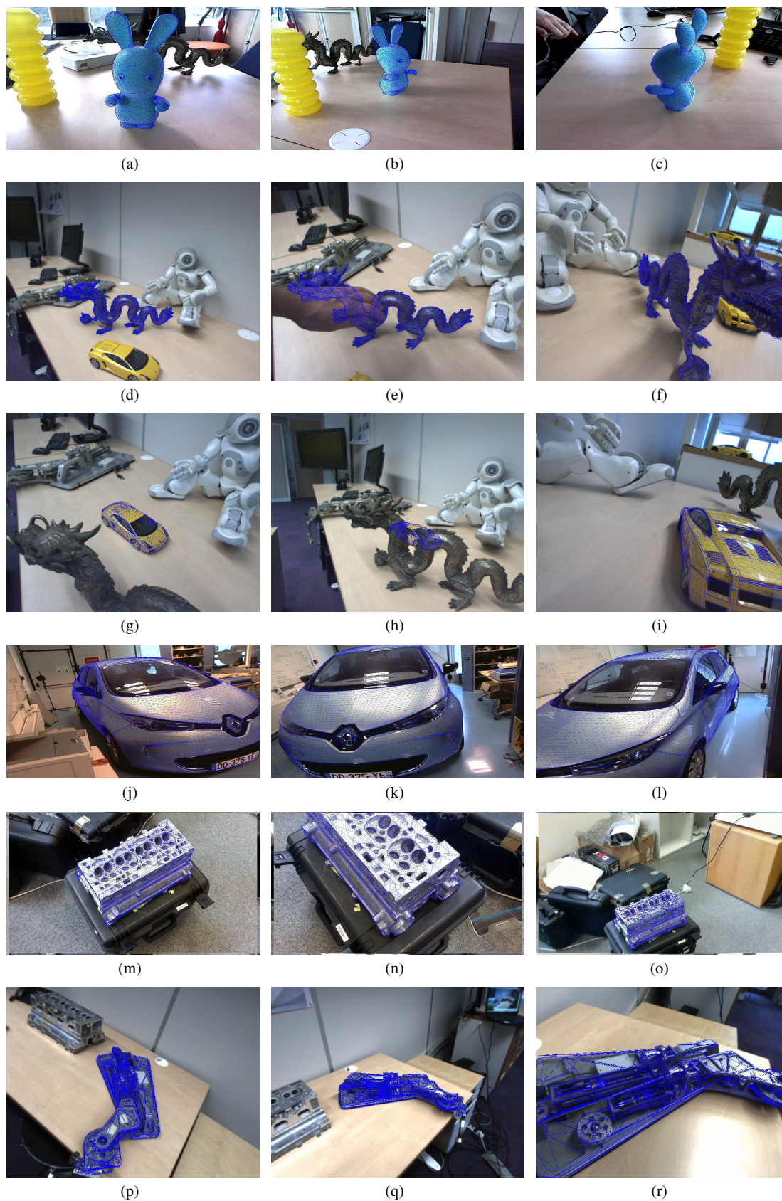
Fig. 24: Accurate localization results on a Raving Rabbid, a dragon, a sport car, a real-sized car, a car cylinder head, and an orthosis with our phDEC-SLAM. Results are similar with rDEC-SLAM and rhDEC-SLAM. The accuracy can be appreciated by the projection of the 3D blue models on the object of interest in the images.
