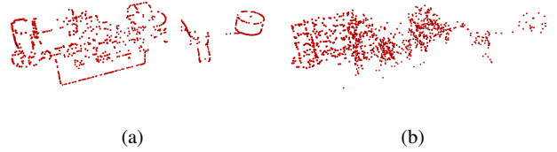
Fig. 10: Set of edgelets extracted with our sampling method on the left and with a random sampling solution on the right.
