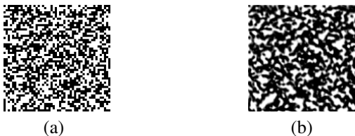
Fig. 1. Example of CDP from Indigo dataset [3]: a) an original random binary image before printing and b) its degraded version by P&D.
