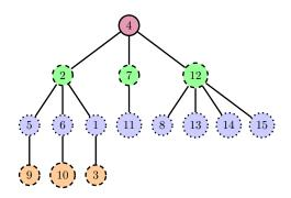
**Figure 3** The Resulting Centroid Decomposition of *G*.
