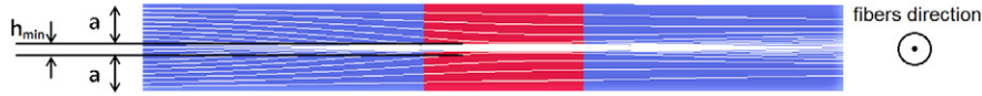
Fig. 6. In-plane flow domain with varying distance h between yarns of fixed thickness a (in red) and varying local permeability. Inter-yarn pores (in blue) are crossed by streamlines (white solid lines), also actively penetrating yarns when h = h_{min} .
