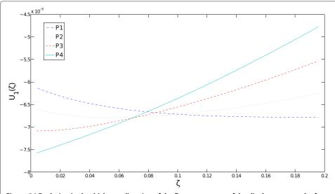
Figure 26 Evolution in the thickness direction of the first component of the displacement at the four locations indicated in Figure 25.
