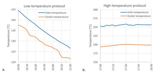
**Figure 6.** Typical averaged inlet and outlet fluid temperatures for the 3 instrumented lines during (a) low-temperature protocol and (b) high-temperature protocol operations.
