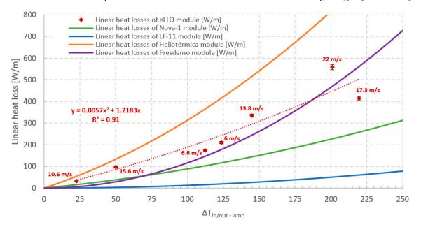
Figure 7. Linear heat losses of Nova-1, LF-11, Heliotérmica, Fresdemo and eLLO modules.
