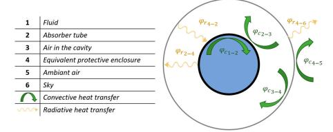
Figure 10. Equivalent geometry of the eLLO receiver for thermohydraulic modeling.
