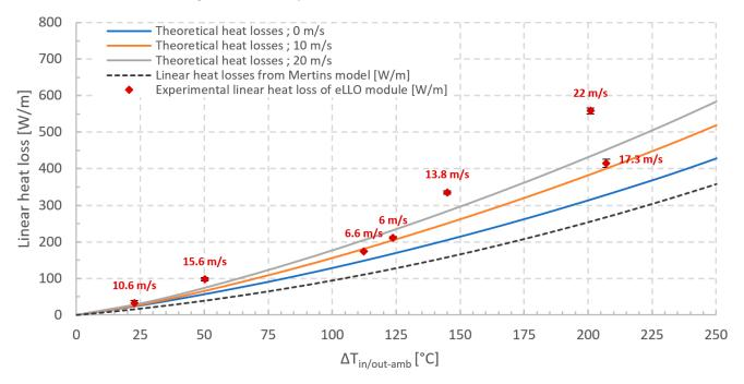
**Figure 14.** Theoretical heat losses of the eLLO receiver as a function of wind speed along with experimental data.
