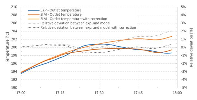
Figure 12. Evolution of the experimental and simulated outlet temperature with and without correction.
