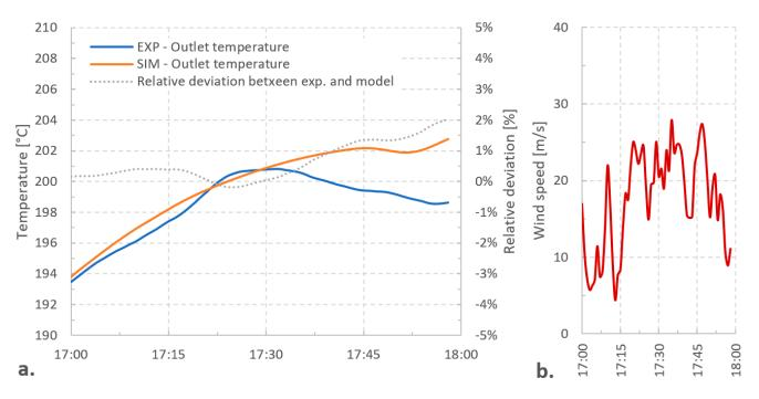
**Figure 11.** (**a**) Evolution of the experimental and simulated outlet temperature and (**b**) wind speed for 01/07/2022.
