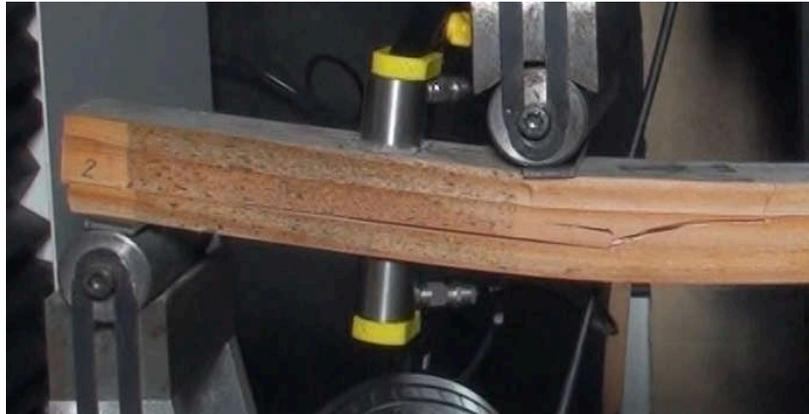
**Figure 9:** Glue joint delamination under load
