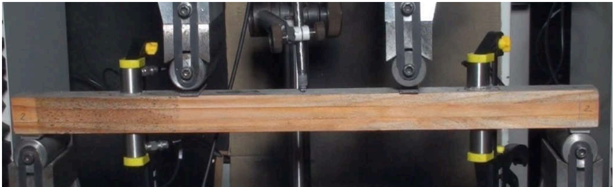
Figure 2: Four points bending experiment configuration
