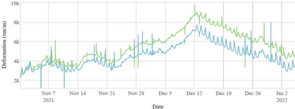
**Figure 6:** Gauges elongation on top and middle lamella of a sample
