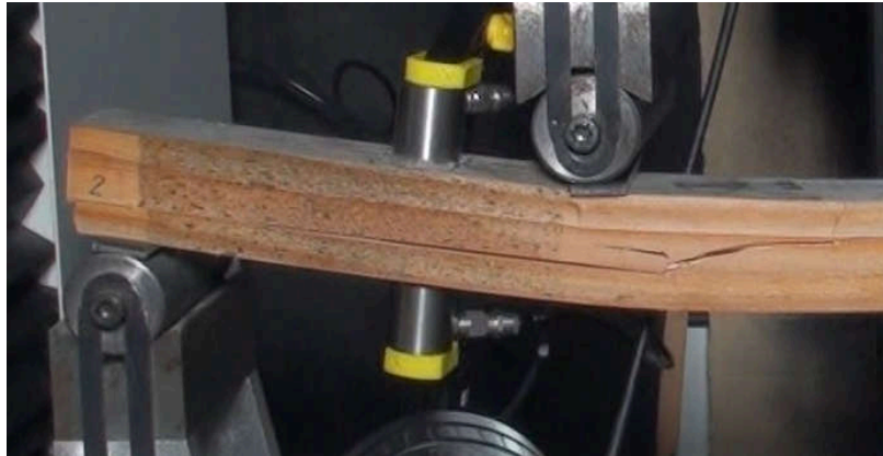
Figure 9: Glue joint delamination under load
