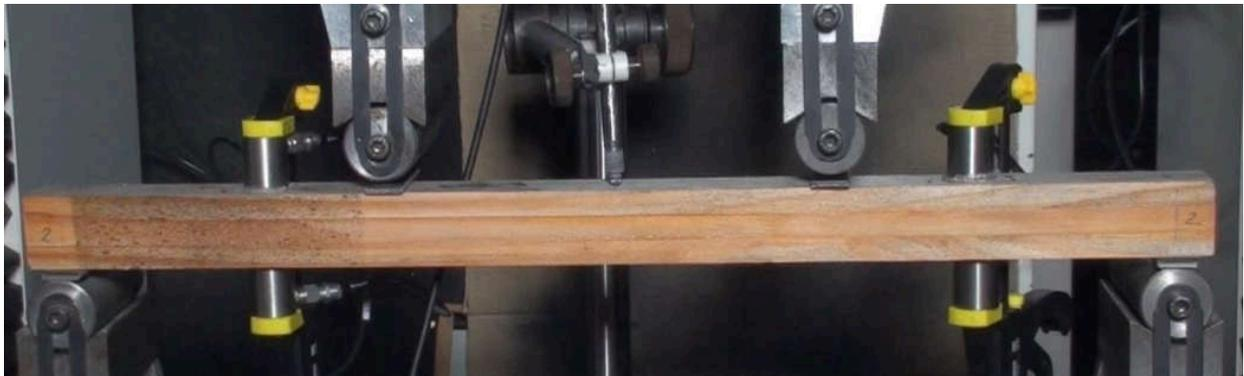
**Figure 2:** Four points bending experiment configuration
