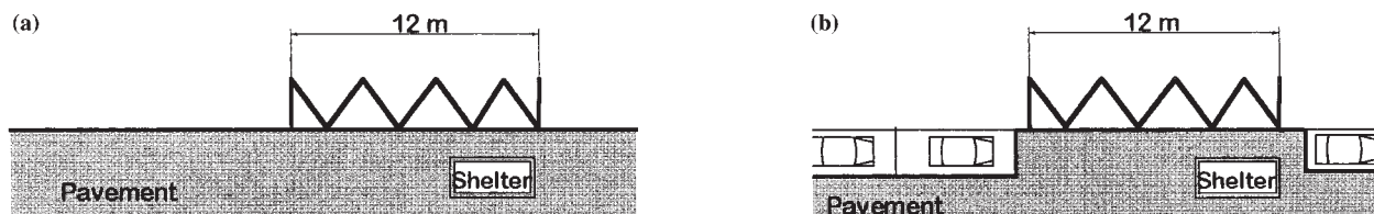
FIGURE 2 (a) Bus stop configuration, on-line; (b) Bus stop configuration, extended bay.
