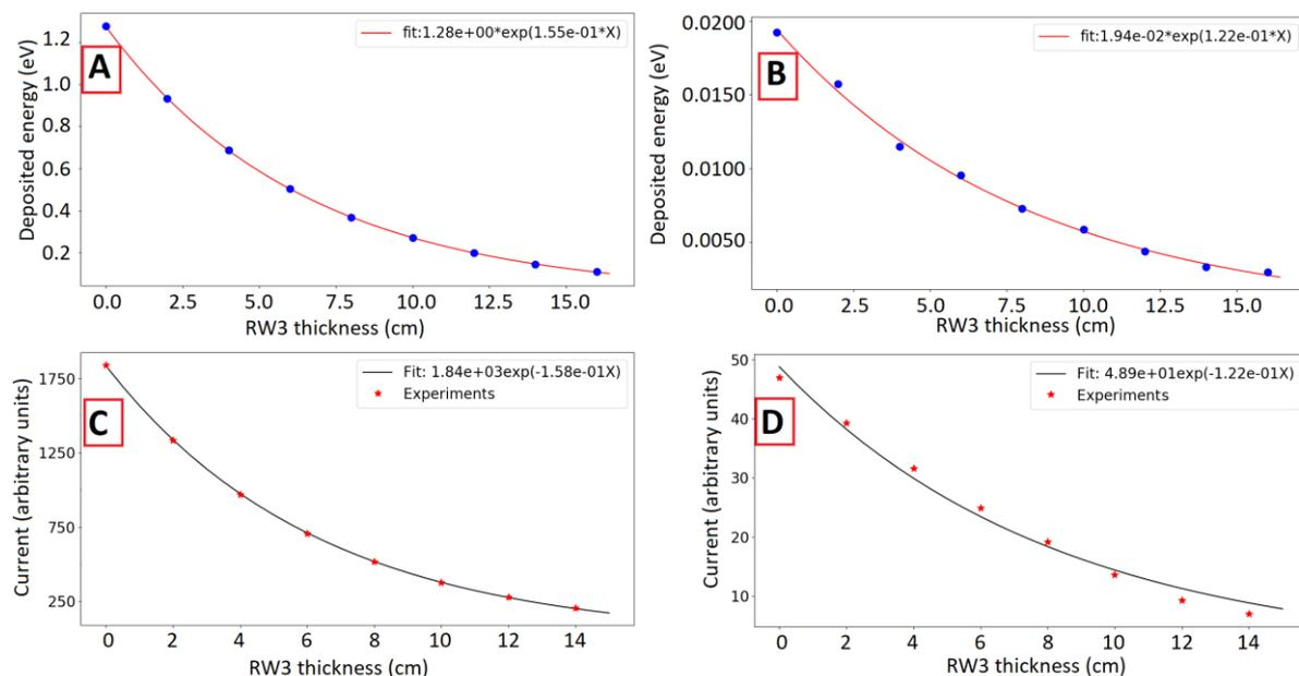
**Figure 9** Detector response as a function of increasing RW3 thickness for the central strip facing a microbeam (A: simulations; C: experimental results), and for an adjacent strip facing an interbeam area (B: simulations; D: experimental results). For the simulations, the deposited energy corresponds to the mean value per incident photon.
