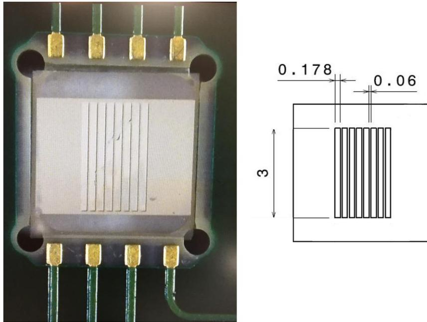
**Figure 2** Image of the prototype of the 8 strips diamond (left) with no guard ring (the backside metallization is visible by transparency). On the right, the diamond's schematic representation where the dimensions are in millimeters.
