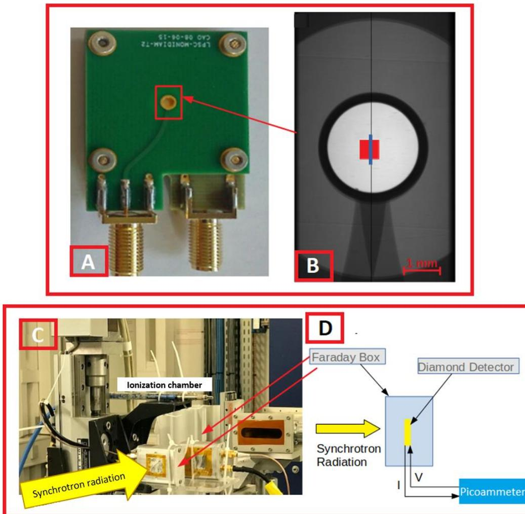
**Figure 1** (A): detector mounted on a printed circuit board (PCB) holder and (B) corresponding detector radiography ( $23 \times 23 \mu\text{m}^2$  pixel size): in red the beam spot ( $0.5 \times 0.5 \text{ mm}^2$ ) and one microbeam in blue ( $50 \mu\text{m} \times 795 \mu\text{m}$ ) are graphically painted. (C): image of the experimental set-up used to test the
