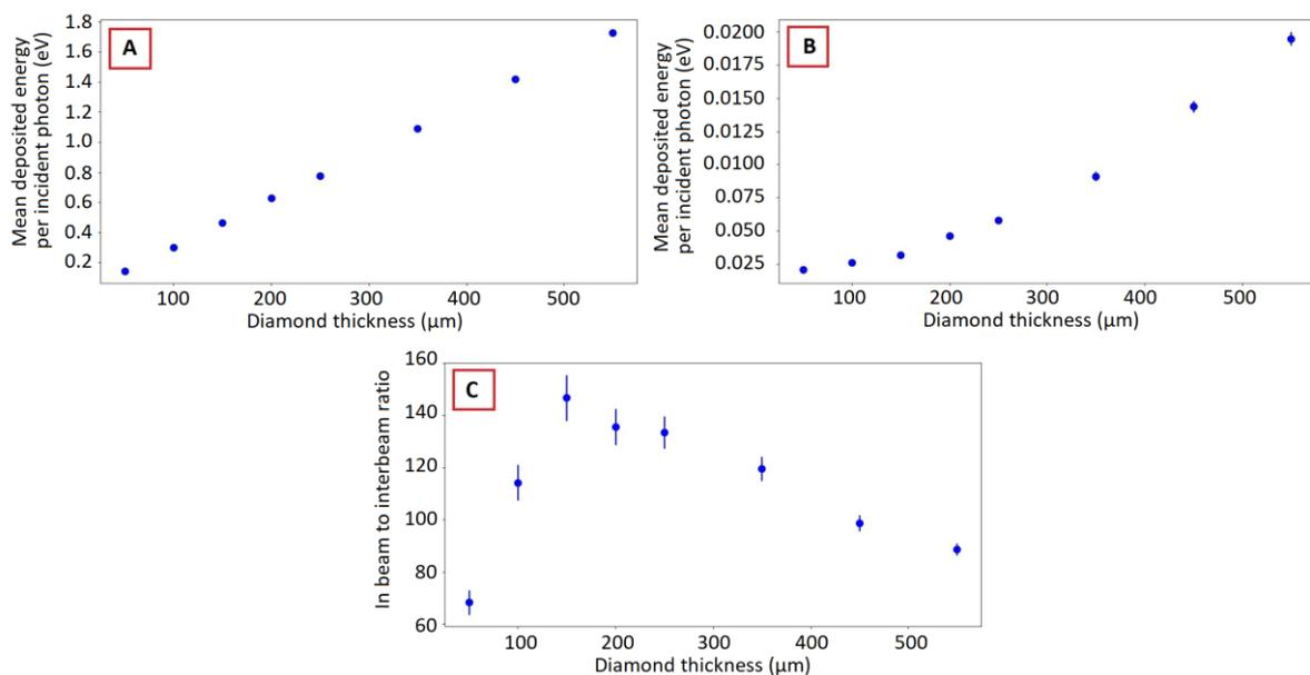
**Figure 4** Calculated diamond's response as a function of the thickness in a strip facing a microbeam (A), and in a strip facing an interbeam (B). Ratio of the average energy deposited in a strip facing a microbeam and in the adjacent strip facing an interbeam (averaged over the two adjacent strips) (C). Calculated for energies < 600 keV.
