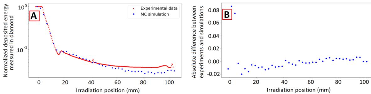
**Figure 10** (A) Simulated (blue points) and measured (red stars) response of a diamond detector strip facing a microbeam during the scan of the anthropomorphic human head phantom. (B) Absolute differences between the experiment and the simulations.
