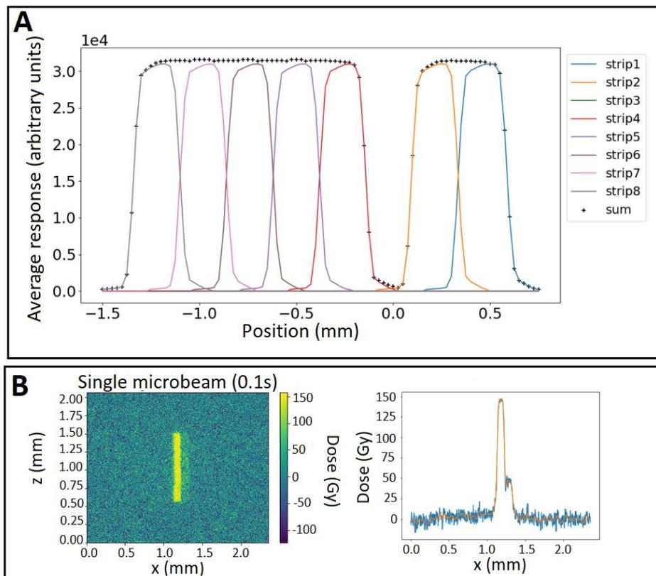
**Figure 8** (A) Result of the horizontal scan with one microbeam. (B) Analysis of the Gafchromic film. On the left, the 2D transverse profile, and on the right, the dose-response along the horizontal axis within the microbeam area.
