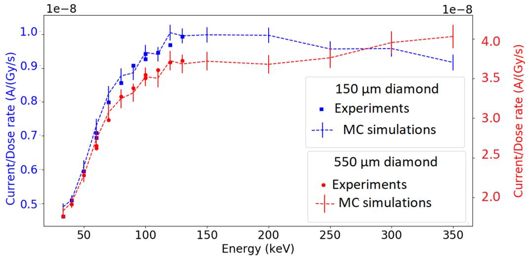
**Figure 6** Results of the response of diamonds normalized by the dose rate in water as a function of energy measurements, and Monte-Carlo simulations.
