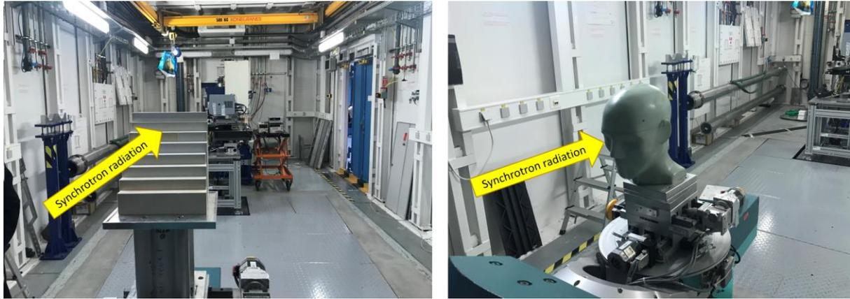
**Figure 3** Photographs of the RW3 staircase phantom with thicknesses ranging from 2 to 16 cm (left), and of the human head phantom (right). The detector was positioned 6 meters behind the phantoms.
