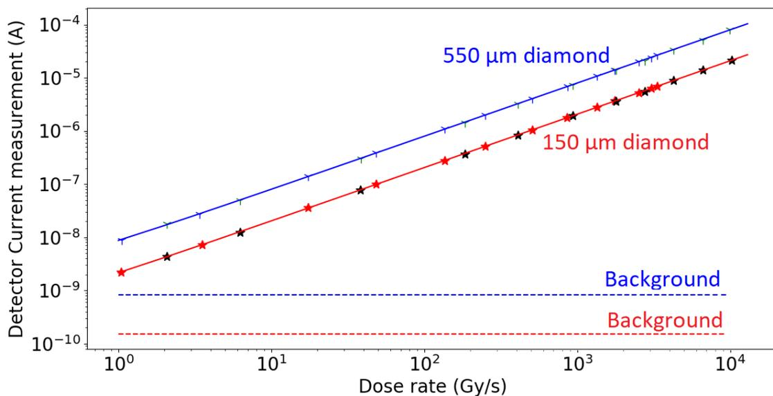
**Figure 7** Responses of the two diamond detectors as a function of the dose rate measured at the MRT hutch, using a filtered polychromatic beam and various PMMA absorbers to reduce the dose rate. For each diamond thickness, two measurement sets were acquired. Horizontal dashed lines correspond to the background current level.
