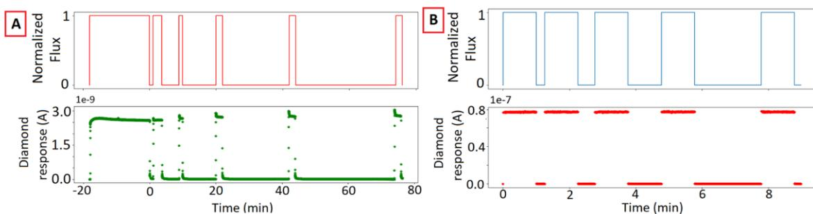
**Figure 5** 550  $\mu\text{m}$  diamond response during 160kV x-ray tube irradiation (A), and 95 keV monochromatic synchrotron radiation (B). During both irradiations, the irradiated area was  $0.5 \times 0.5 \text{ mm}^2$ .
