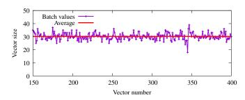
Figure 1: Oscillation of batch sizes for a L2 forwarding function that processes a constant 5 Gbit/s traffic.
