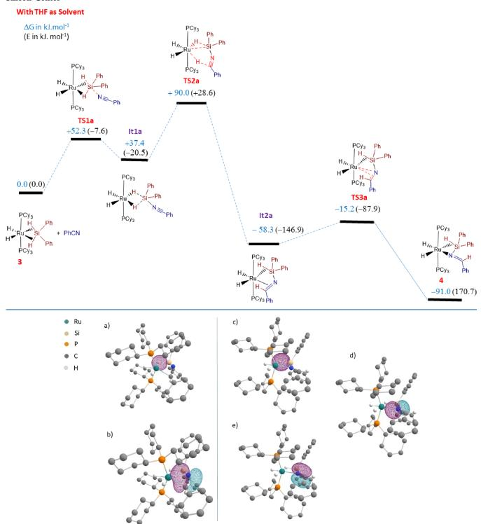
Figure 5. pNLMO representation at the left: It2a intermediate (a)  $Ru(\eta^2\text{-SiH})$  and (b)  $Ru(\eta^2\text{-C=N})$ ; right: complex 4 (c)  $Ru(\eta^2\text{-SiH})$ , (d)  $Ru(\kappa N\text{-}N\text{=C})$  and (e) N=C bond. hydrogen atoms attached to carbon atoms are omitted for clarity except for the imino fragment.
