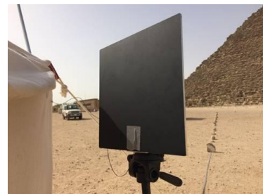
View of the tent positioned 175 m from the North face, the infrared camera and the calibration plate installed in its field of view.
