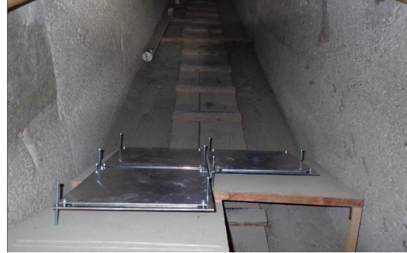
Photo of test emulsion plates installed in the descending corridor during missions from January to April 2016.
