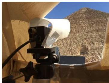
View of the tent positioned 175 m from the North face, the infrared camera and the calibration plate installed in its field of view.
