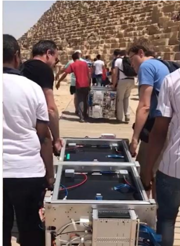
Sébastien Procureur (blue T-shirt) and the CEA team will position the Degennes, Charpak and Joliot telescopes inside the pyramid to investigate the SP-NFC.
