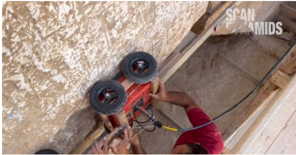
Data acquisition with ground-penetrating radar.
