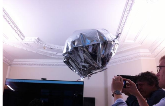
At this meeting, Jean-Baptiste Mouret, a robotics specialist at INRIA 213 Strasbourg, presented a prototype of an inflatable airship that could be introduced into a cavity through a 3cm diameter borehole, with a view to possible exploration.
