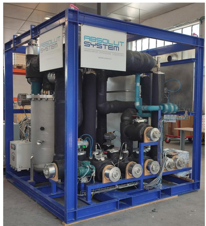
Fig. 10. Cryogenic skid, being tested.
