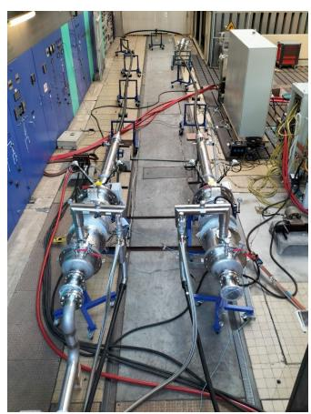
**Fig. 12.** Cable type test loop installed at the SNCF Railway Test Agency (SNCF-AEF), including two terminations and a joint.
