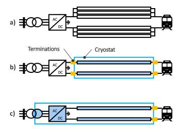
**Fig. 13.** a) Conventional solution, b) Montparnasse-Vouillé demonstrator (TRL 6-7), c) Lab prototype (TRL 4) with a superconducting transformer and a power electronic converter operating at cryogenic temperature.
