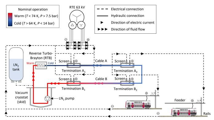
Fig. 9. Architecture of the cooling system connected to the HTS cables, in nominal operation.
