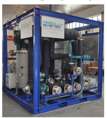
Fig. 10. Cryogenic skid, being tested.
