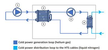
Fig. 8. RTB cooling machine operating principle.
