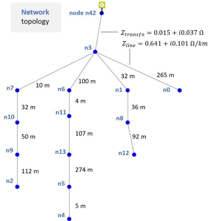
Fig. 5 - Low-voltage network adapted from the SimBench dataset.
