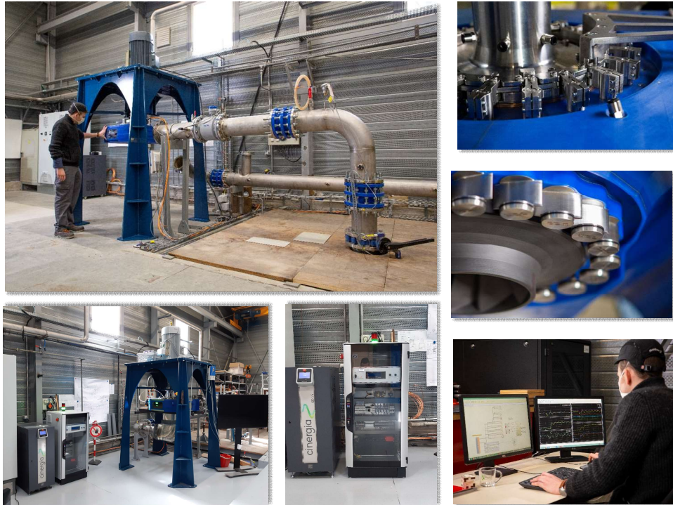
Figure 4-1 (top left and bottom left) SuperGrid Institute's HydroPHIL platform architecture dedicated to real time simulations. (upper right) Actuator of the PSP: namely the guide vane operating ring, and inside of the turbine, runner, and wicket gates (bottom centre) ESS on the right and grid emulator on the left
