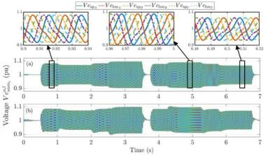
Figure 11: Voltage of the equivalent capacitor of the MMC arms  $v_{c_{sum i}}^{u,l}$  (a) – NEBC, (b) – EBC
