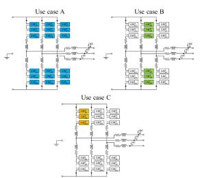
Figure 8: MMC with energy storage devices in all arms for use case A, only in one phase (leg B) for use case B and only in one arm for use case C
