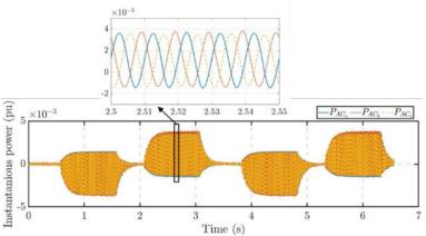
Figure 16: Instantaneous active power for NEBC with PR-CCSC
