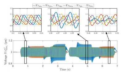
Figure 19: Voltage of the equivalent capacitor of the MMC arms  $v_{C_{sumi}}^{u,l}$
