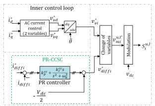
Figure 14: Inner control loop for NEBC using a PR-CSCC
