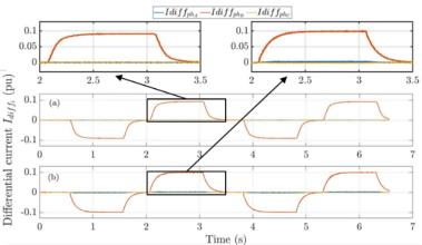
Figure 15:  $i_{diff_i}$  in use case B (a) – EBC, (b) – NEBC with PR-CSCC
