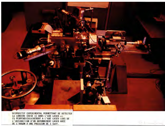
Figure 1. (left) Picture of the first spectrometer used by Anne L’Huillier and coworkers to measure their first published HHG spectrum (right).
