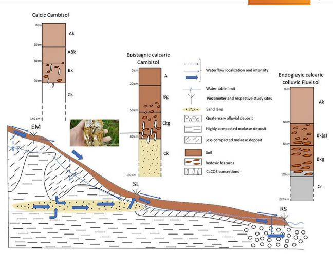
FIGURE 13 Conceptual scheme of the different types of water pathways identified in the soils of the Molassic Hills.
