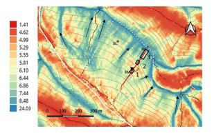
**FIGURE 14** Beven index determined with a 5 m digital elevation model (DEM). The contour lines are spaced at 5 m ( $\mathbf{\nabla}$ : position of embankment [EM] point, |1||2||3|: delimitation of areas on transect described in Figures 11 and 12).
