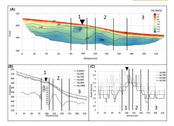
**FIGURE 11** Velocity of P-waves ( $V_p$ , m/s) determined by seismic prospection along the embankment-riverside (EM-RS) transect, as a surrogate for layer compactness, versus topography (A and B) and versus depth (C) ( $\mathbf{\nabla}$ : EM point, 111: rise of compact material above EM point, 121: rise of compact material below the EM point, 131: increase in soil thickness with quick transition to compact material).
