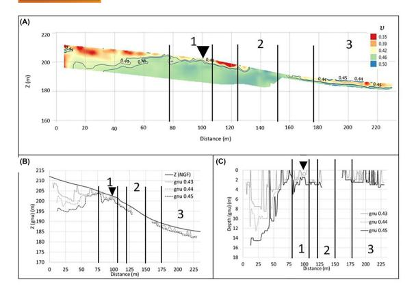
**FIGURE 12** Poisson ratio versus topography (A and B) and versus depth (C) determined by seismic prospection along the embankment-riverside (EM-RS) transect ( $\mathbf{\nabla}$ : EM point, 11||2||3|: areas of high v associated with the rise of compact material described in Figure 11).
