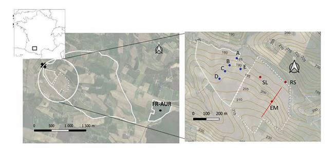
**FIGURE 1** Study plots inside the watershed. (X: outlet of the watershed, **FR-AUR**: meteorological station; A–E: toposequence points; RS, riverside; SL, sand lens; EM, embankment. The redline indicates the position of the geophysical transect). Plot 1: continuous white line, plot 2: dotted white line. The contour lines are spaced 5 m apart.
