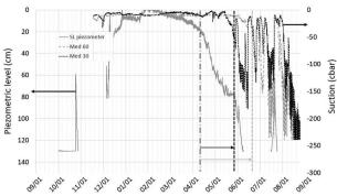
**FIGURE 10** Suction head monitoring (Med 30 and 60, median values at 30 and 60 cm, respectively) of the sand lens (SL) point versus the piezometric level during a complete hydrological cycle. The black and gray arrows on the dotted vertical lines show the temporal shift between the lowering of the piezometric level and the drop in suction.
