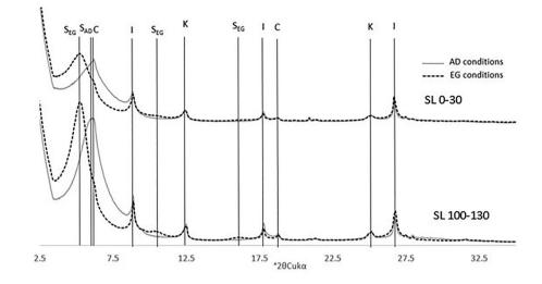
**FIGURE 4** Diffractograms of the clay fraction with peaks characteristic of clay minerals for sand lens (SL) point at 30 and 130 cm depth. S, smectite; C, chlorite; I, illite; K, kaolinite
