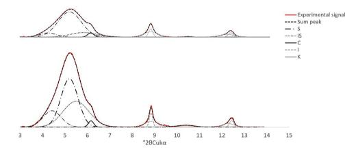
FIGURE 5 Decomposition of X-ray diffraction (XRD) patterns for sand lens (SL) samples in ethylene glycol (EG) treatments. S, smectite; IS, mixed interlayered minerals; C, chlorite; I, illite; K, kaolinite
