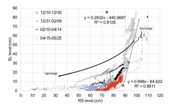
**FIGURE 9** Relationship between sand lens (SL) and riverside (RS) piezometric levels during the saturation and discharge phases of the SL piezometer, from December 10, 2020 to May 25, 2021. Linear regressions: evolution of the piezometric level during discharge between (A) 75 and 85 cm depth, and (B) deeper than 85 cm.
