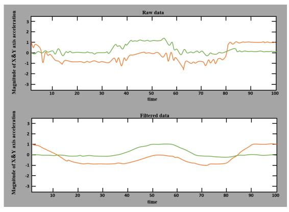
Figure 2. Comparison of acceleration before and after data denoising
