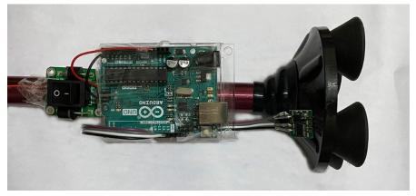
Figure 4. Instrumented walking stick.
