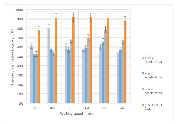
Figure 6. Comparison of classification result from different sensors' data at six walking speeds.
