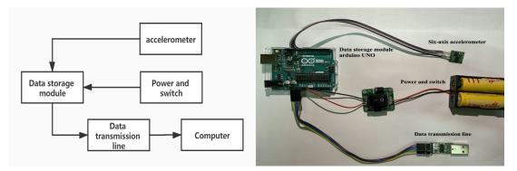
Figure 1. Terrain recognition device based on accelerometer
