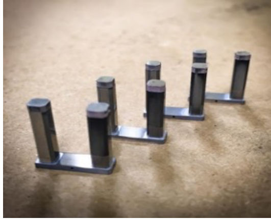
FIG 4. TESI-produced flight-like SKD-based couples.
