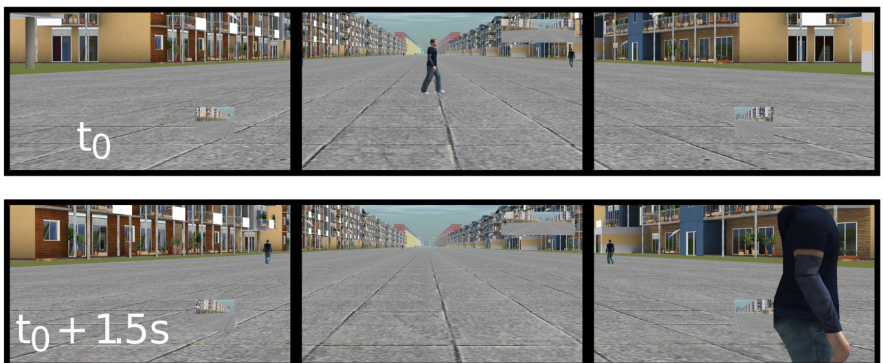
Fig 5. Screenshots of the three monitors during the experiment. Note. The two screenshots illustrate participants' view during a crossing situation at a time interval of 1.5 s. In this situation, the vehicle was driving 20 kph (vehicle speed = 20 kph). The pedestrian was crossing the street from left to right (pedestrian position = left) at 5.5 kph (pedestrian speed = 5.5 kph) facing the vehicle (orientation = face) with an angle of \text{Pi}/3 (angle = \text{Pi}/3 ). The pedestrian passed in front the vehicle (order = first), respecting a safety margin of 1.5 m (margin = 1.5 m).
