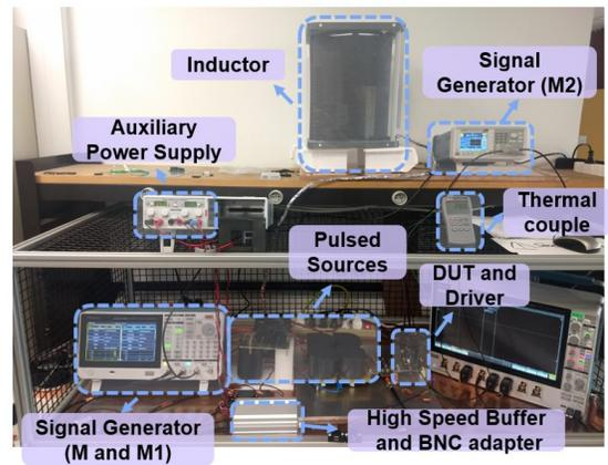
Fig. 2. DST bench used for switching characterization.
