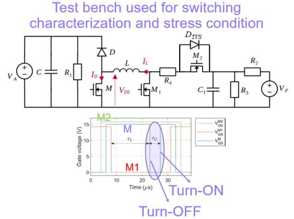
Fig. 1. Electrical schematic of double source test.
