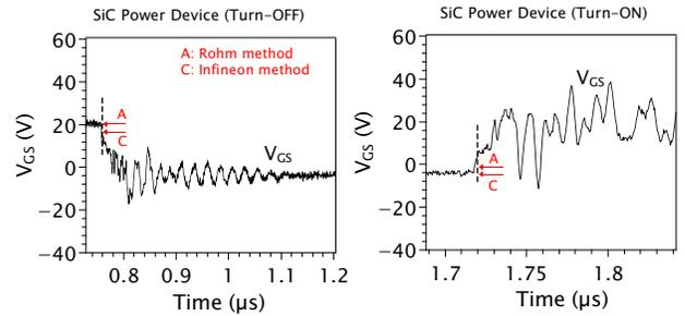
Fig. 8. Waveforms of gate-source voltage during turn-OFF and turn-ON events. The red arrows correspond to the initial integration limit for the method A and C.
