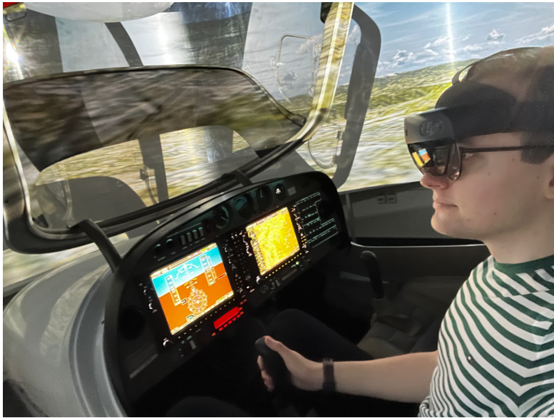
Figure 2: Picture of a pilot who tests the interaction with augmented en-route flight information through a mixed reality headset in a high-fidelity Diamond DA 40 simulator.
