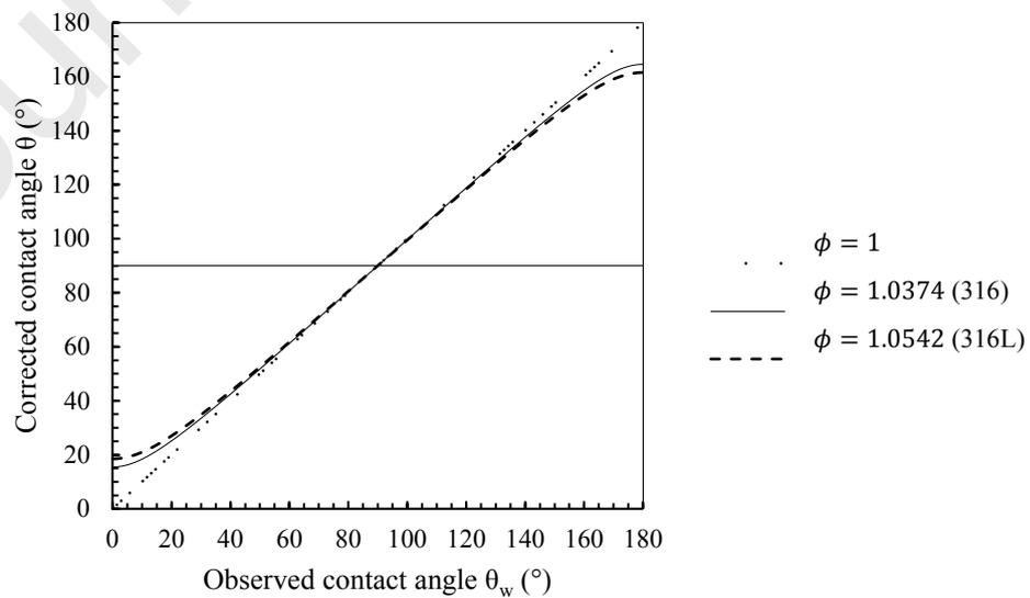
Figure 7 Roughness effect following the Wenzel equation considering maximal values of  $\phi$  parameter for AISI 316 and AISI 316L surfaces
