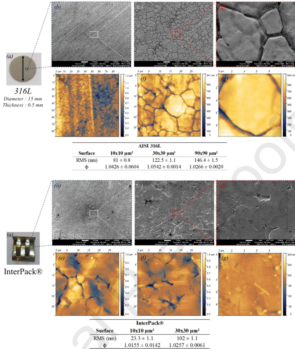
Figure 3 Surface characterization of AISI 316, 316L and InterPack® element: (a) sample picture; (b,c,d) SEM-FEG observations with magnification of  $\times 100$ ,  $\times 1000$  and  $\times 10000$ , respectively; (e,f,g) AFM observations; and table of AFM measurement results
