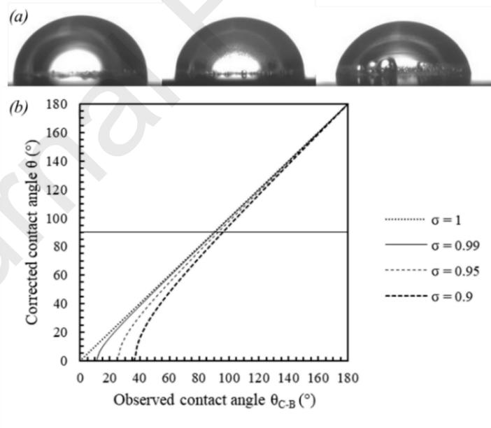
Figure 9 (a) picture of trapped bubbles, (b) correction of the observed contact angle through the Cassie-Baxter equation for various arbitrary wetted fraction
