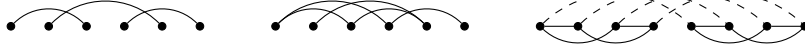
FIGURE 7. A strict queue; a queue; and a 2-queue-layout of the cube, partitioned in solid and dashed edges.
