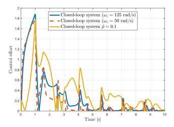
Figure 7. Time evolution of the control effort for system (10)-(12) in closed-loop in presence of a 0.05s delay in the actuation path using the control law (51) with  $\tilde{\rho}=0.2$  and the filtered control law introduced in Theorem 8 for different filters
