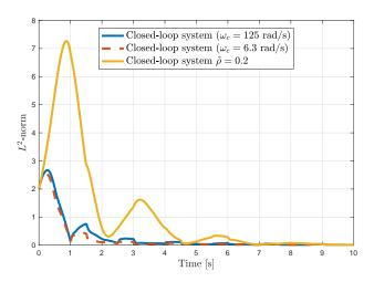
Figure 6. Time evolution of the  $L^2$ -norm of the system (10)-(12) in closed-loop in presence of a 0.05s delay in the actuation path using the control law (51) with  $\tilde{\rho}=0.2$  and the filtered control law introduced in Theorem 8 for different filters
