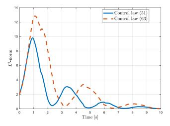
Figure 8. Time evolution of the  $L^2$ -norm of the system (10)-(12) in closed-loop using the control law (51) (with  $\tilde{\rho}=0$ ) and using the control law (63)
