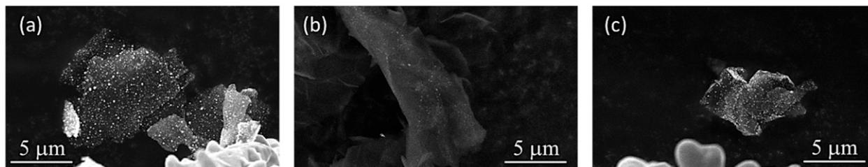
**Figure 6.** SEM micrograph of an (a.) graphene sheet with Cu(O) nanoparticles without HN pre-treatment, (b.) graphene sheet with Cu(O) nanoparticles without HN pre-treatment and after 10 s of ultrasonic treatment, (c.) graphene sheet with Cu(O) nanoparticles with HN pre-treatment and after 10 s of ultrasonic treatment.
