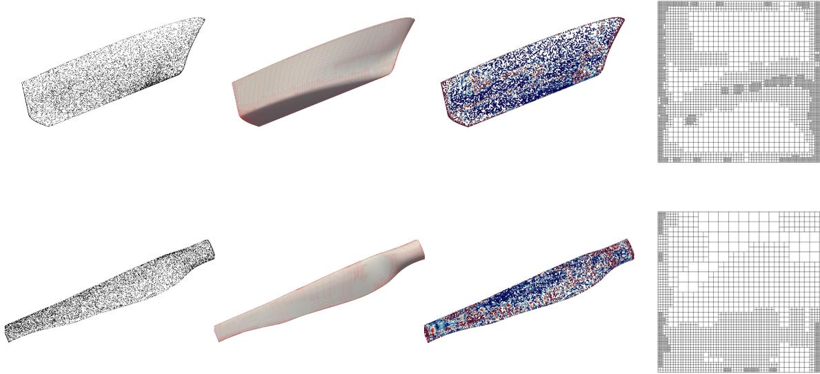
**Fig. 22:** The point cloud, the hierarchical spline model reconstruction, the scaled error distribution and the hierarchical mesh for a ship hull (top) and a wind turbine (bottom) using the BIDGCN parameterization with bidegree  $(5, 2)$ .
