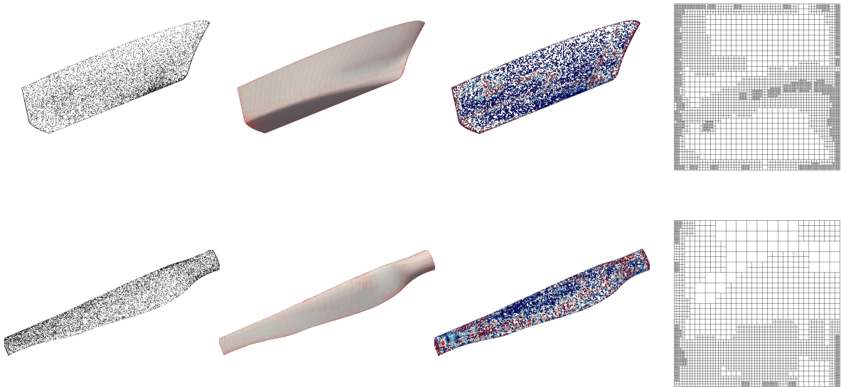
Fig. 16: The point cloud, the hierarchical spline model reconstruction, the scaled error distribution and the hierarchical mesh for a ship hull (top) and a wind turbine (bottom) using the BIDGCN parameterization with bidegree (5,2).
