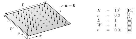
**Fig. 6**: Geometry and parameters for the example of a unit-square plate with a distributed vertical load  $f_z$  given by Eq. (57). The displacements are fixed on all edges.
