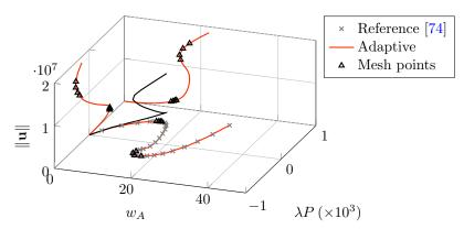
Fig. 19: Projection the adaptively refined result from the commonly used  $\lambda P, w_A$ -space [74] onto the displacement norm  $\|\mathbf{u}\|$ . The solid lines correspond to the results obtained by the adaptively refined mesh, the triangular markers correspond to points of which the mesh is provided in Fig. 20 and the cross-markers indicate the result from [74].
