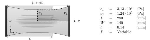
**Fig. 21**: Geometry and parameters for the wrinkling problem. The boundary  $\Gamma_1$  is free, the boundary  $\Gamma_2$  is fixed in x and y direction and rotations around the y-axis are fixed, the boundaries  $\Gamma_3$  and  $\Gamma_4$  have symmetry conditions applied.
