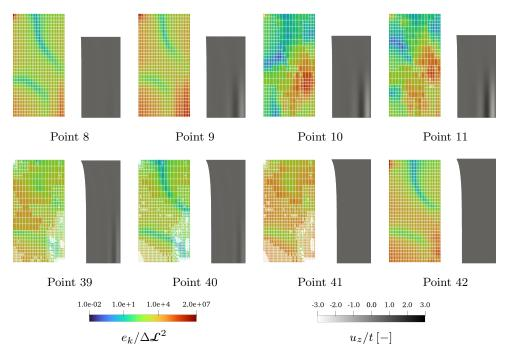
**Fig. 23**: Normalized element errors (left) and the normalized out-of-plane deformation (right) for the wrinkling benchmark plotted on the undeformed geometry with the corresponding elements.
