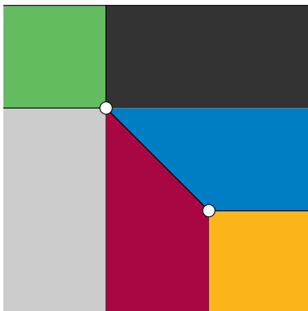
Figure 8: Multi-patch decomposition of a simple domain into six patches. The domain has two EVs in the interior (valence 3 and 5) and no boundary EVs.
