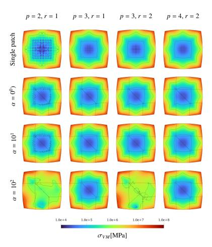
Figure 16: Von Mises membrane stress fields for the single patch, unstructured splines and penalty-coupled multipatch paraboloid from Section 4.2 and Fig. 13 with  $64 \times 64$  elements per patch. The results are provided for different combinations of degree p and regularity r. The color bar represents the stress and the contours are plotted for stress levels  $\sigma_{VM} \in \{10^5, 10^6, 10^7\}$  [MPa].
