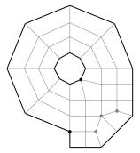
(a) A simple mesh with boundary edges in black and interior edges in gray. The boundary extraordinary vertices (bEVs), i.e. the vertices on a boundary with valence  $v \ge 3$  are denoted by a black circle and the interior extraordinary vertices (iEVs), i.e. interior vertices with valence  $v \ge 4$ ,  $v \ne 4$  are denoted by gray circles.
