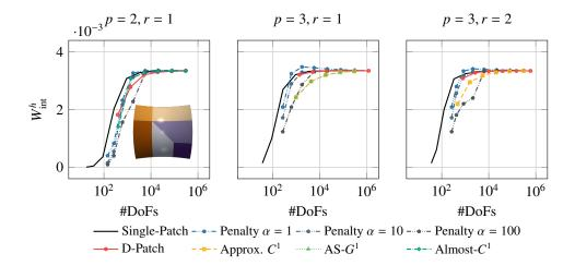
Figure 12: Bending energy norm  $W_{\text{int}}^h = \frac{1}{2} \mathbf{u}_h^{\mathsf{T}} K_h \mathbf{u}_h$  for the hyperboloid geometry from Fig. 10 with a patch segmentation as in Fig. 8. The results are presented for different combinations of the degree p and regularity r for all unstructured spline constructions. In addition, the results for a penalty method with parameter  $\alpha \in \{1, 10, 100\}$  are provided for comparison.
