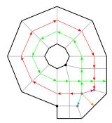
(b) Illustration of the interface tracing procedure. From each EV all outgoing edges are traced as illustrated until another EV or a boundary is hit.
