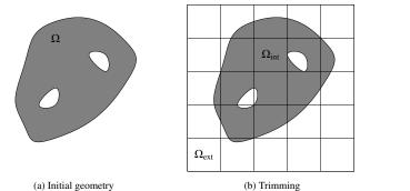
Figure 3: Given an initial geometry  $\Omega$  (a), trimming (b) uses the curves of the boundary of the original geometry to define the interior domain  $\Omega_{int}$  and the exterior domain  $\Omega_{ext}$ . An alternative approach for modelling the domain is to use domain segmentation (c). Here, the domain is decomposed into several patches  $\Omega_i$  which together define the full domain  $\Omega$ .
