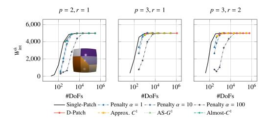
Figure 13: Bending energy norm  $W_{\text{int}}^h = \frac{1}{2} \mathbf{u}_h^{\mathsf{T}} K_h \mathbf{u}_h$  for the paraboloid geometry from Fig. 11 with a patch segmentation as in Fig. 8. The results are presented for different combinations of the degree p and regularity r for all unstructured spline constructions. In addition, the results for a penalty method with parameter  $\alpha \in \{1, 10, 100\}$  are provided for comparison.
