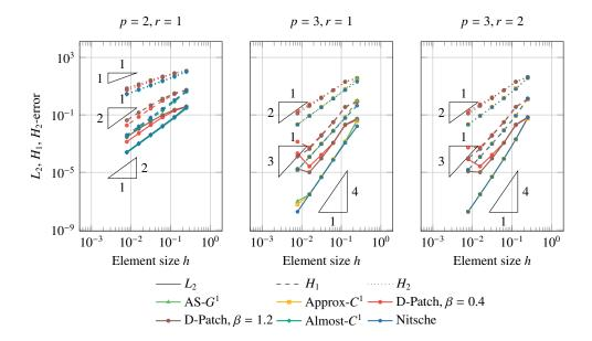
Figure 9: Errors for the AS- $G^1$ , Approx.  $C^1$ , D-Patch and Almost- $C^1$  construction for the biharmonic problem on the domain in Fig. 8. The  $L_2$ ,  $H_1$  and  $H_2$  errors with respect to the analytical solution are plotted with different line styles in the top row. Furthermore, all results are plotted against the element size h and the expected convergence rates are given by the triangles.
