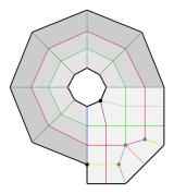
(c) Result of interface tracing from all the EVs. Every patch is now bounded by a a set of boundary and traced interface curves. All patch corners are corners where a traced interface and/or a boundary edge form a corner. Along the hole, different patches are indicated with different shades of gray. In the part bottomright of the hole, every face forms a patch, since all traced curves denoted by colors intersect with other traced curves.
