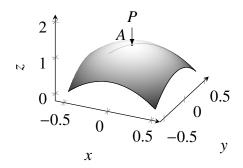
Figure 11: Elliptic paraboloid shell geometry with coordinates  $\mathbf{r}(\xi_1,\xi_2) = \begin{bmatrix} \xi_1 & \xi_2 & 1 - 2(\xi_1^2 + \xi_2^2) \end{bmatrix}$ ,  $\xi_1,\xi_2 \in [-1/2.1/2]$ . On the corners of the domain, the vertical displacements are set to zero  $u_z = 0$  and one corner is fixed in-plane as well. Furthermore, a point load with magnitude  $P = 10^8 t$  is applied in the middle of the geometry.
