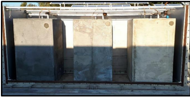
Figure 2 Picture of the IMCB-ODE experimental device before immersion, containing 3 low-pH concrete blocks.
